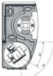
2ª Posición de redonda • Lona entre 25° y 70° aprox. 2nd position of arm support • Canvas between 25° and 70° approx.
